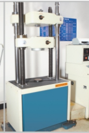
Universal Testing Machine (Tensile, Yield Strength...etc) 拉伸試驗機
